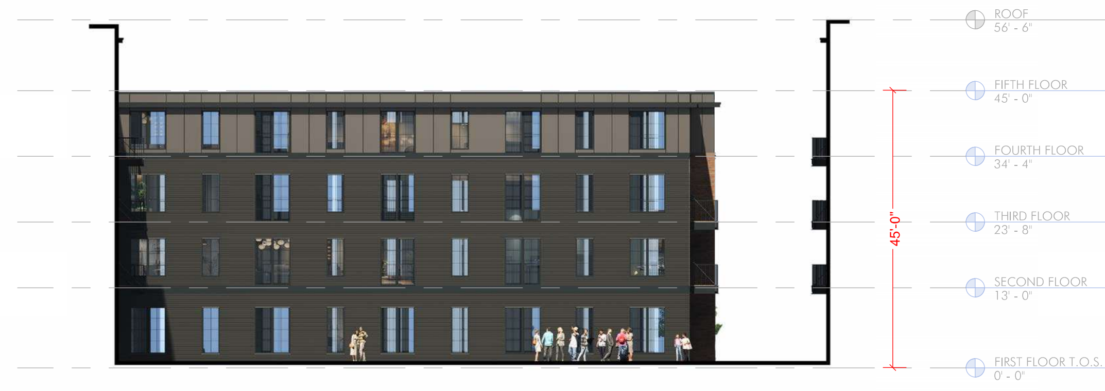
2 NORTH ELEVATION - COURTYARD 1/16" = 1'-0"
