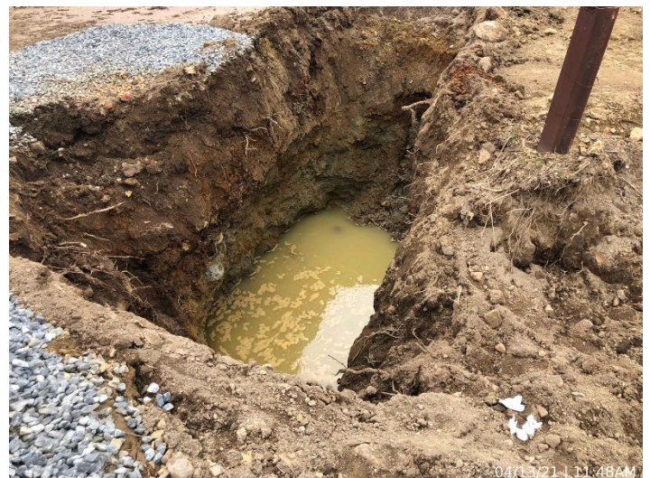
Photo depicts the test pit to determine depth of groundwater.
